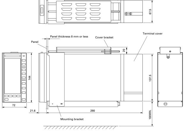
Note) The distance between other instruments and low end of PDA shall be more than 100mm.
