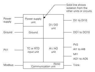
(Note) The communication unit is not isolated from the Al/AO unit when using T-link.
